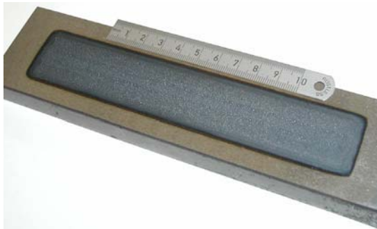
Figure 10 Heat treatment of carbon steel with 2,5 kW HPDL and scanning optics, track width: 27 mm
