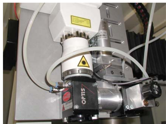
Figure 1 4 kW HPDL laser head with external scanning optics
