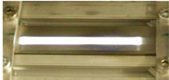
Figure 13 Heat treatment of steel sheet with scanned laser beam, width: 85 mm, Laser: 2,5 kW HPDL
